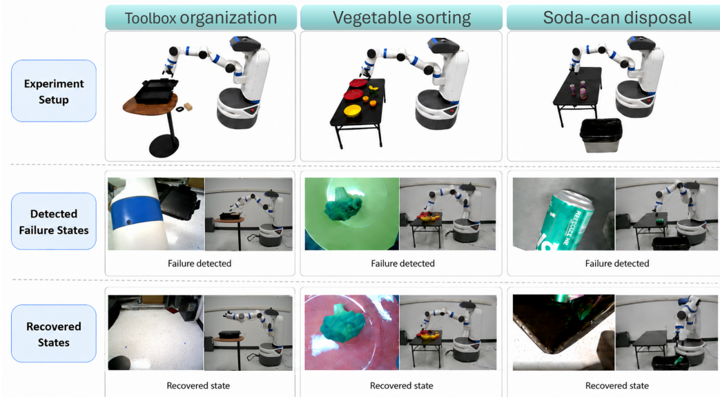
Figure 3: Physical experiments setup. Columns show the three evaluation tasks: organizing the toolbox; sorting vegetables; and soda-can disposal. Rows show the initial experiment setup, example task progress, a detected failure state from the VLM failure analyzer, and the recovered state after residual correction. The examples illustrate that the recovery descriptor must be task-specific and stage-specific: recovering a dropped cable or box, correcting an object-category placement error, and completing soda-can disposal require different active entities and reward components.
